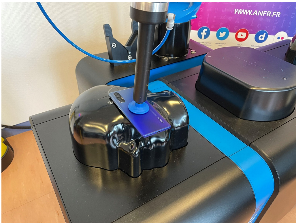
B2. A probe positioned above a phone mounted on a phantom. ANFR photograph of the positioning beneath the probe.
