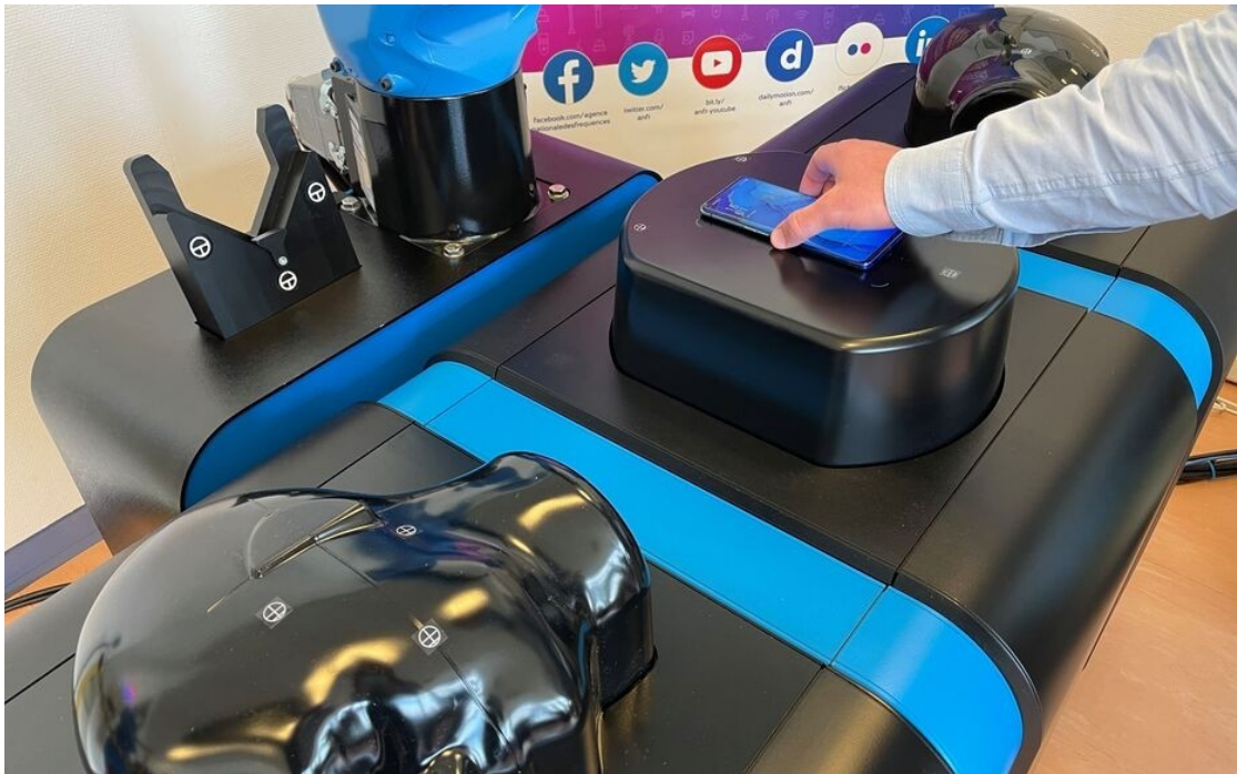
B1. Phone placed on a measurement platform alongside anatomical phantoms. Photograph supplied for this dossier; ANFR laboratory surroundings are visible.
