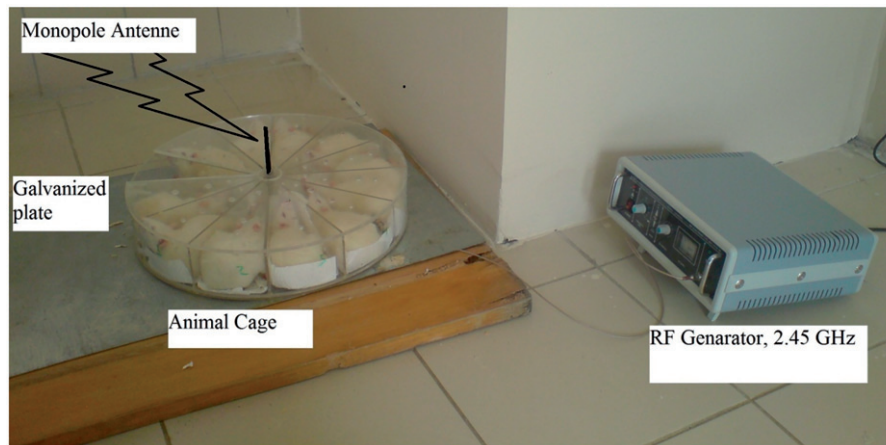
Figure 1. Electromagnetic field exposure system.
