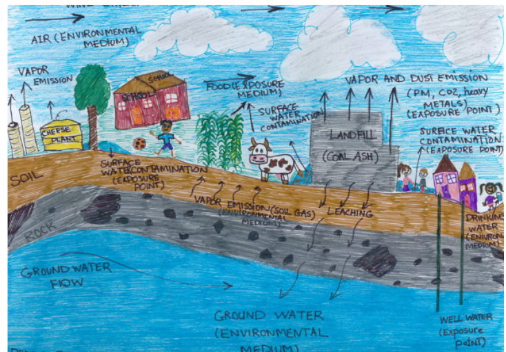
Figure 1 An example of a contamination pathway conceptual model
