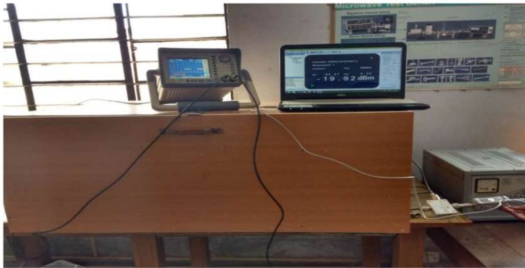
Fig. 1. A. Layout of exposure setup. B. Schematic design of exposure setup for microwave exposure of rats with all apparatus used. The transmitter and receiver antenna (patch) is at distance R from the rat cage.
