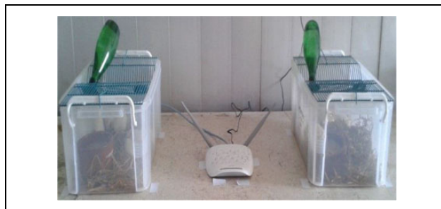
Figure 1. Exposure system design (a standard 2.45-GHz radio frequency source with 802.11.b mode and WPA2 network protection).
