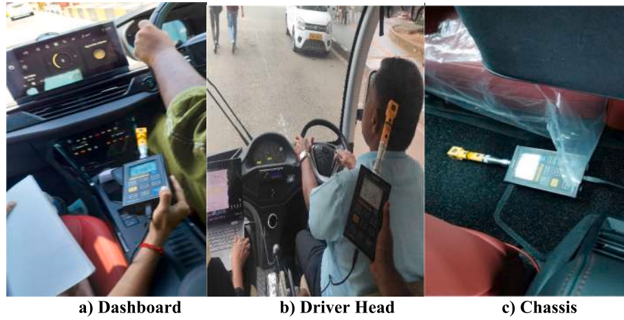
Fig. 2.6. Pictures taken during B field measurement at different positions while driving.
