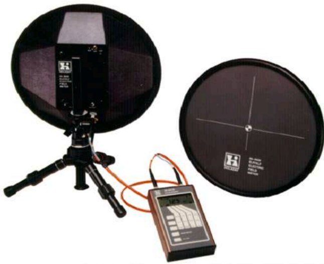
Fig. 2.3. Electric field meter.
