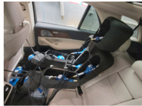
Dummy with measuring probes in the back of an electric car
