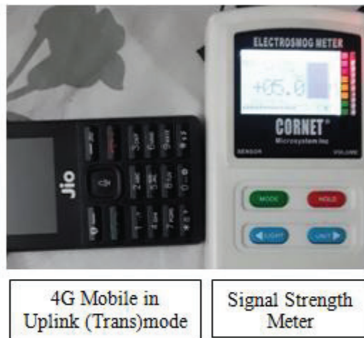
Fig. 3. RF strength measurement
