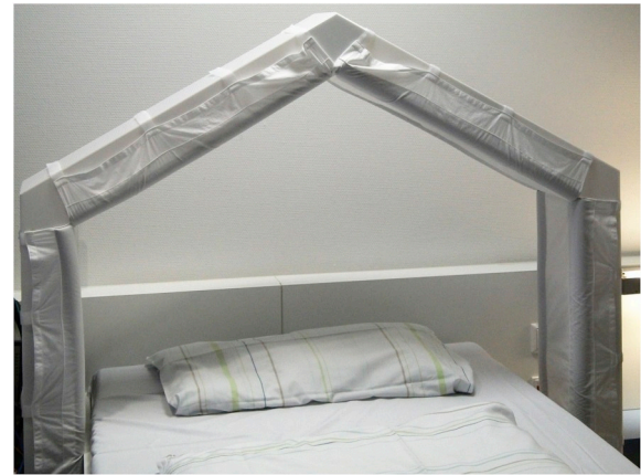
Fig. 2. Structure containing the antennas. Six commercially available Wi-Fi patch antennas were positioned every 60° along a circle of 0.6 m radius in order to meet the requirement of an almost uniform exposure of the head regardless of the subject's position.
