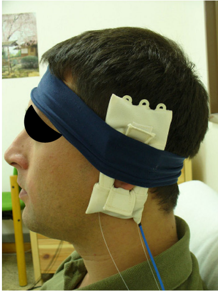
Fig. 1. Position of the antenna. The antenna was fixed to the left side of a subject's head using a common cloth headband.
