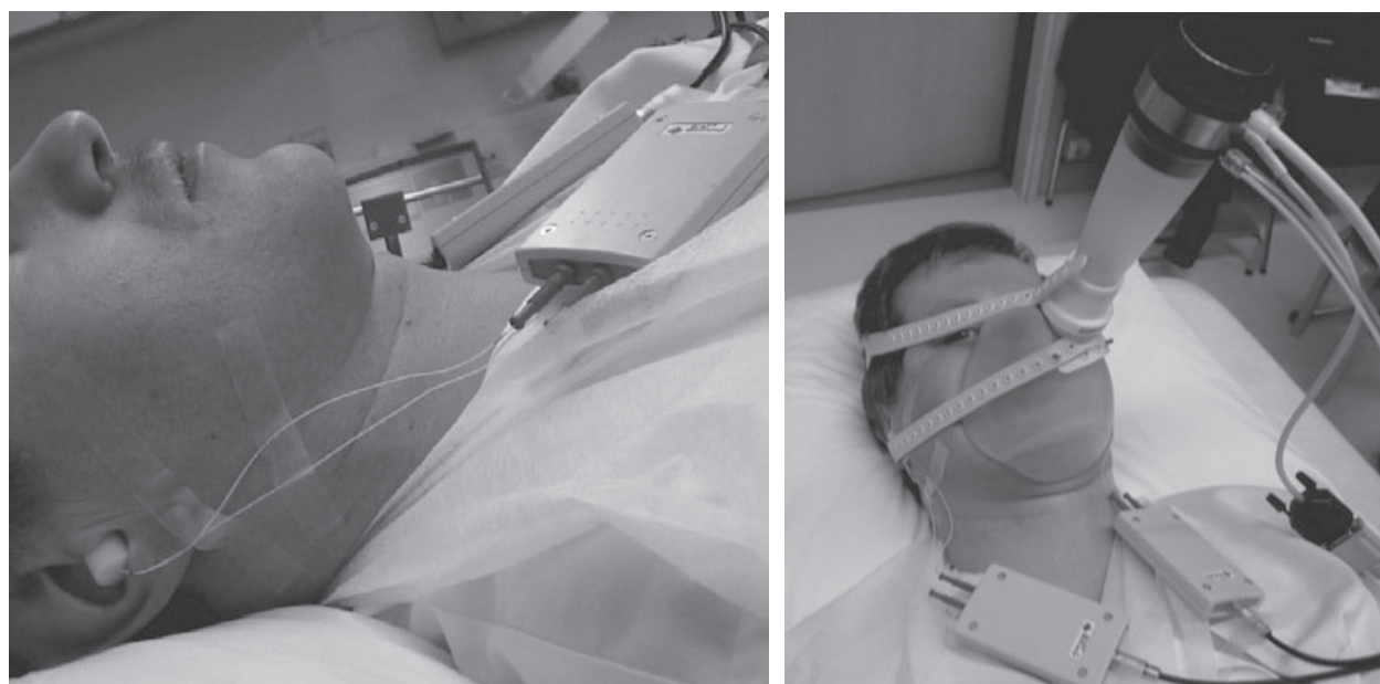
Figure 1 Set-up for head area instrumentation. Small-sized NTC thermistors were applied to ear canals through ear plugs (left figure), thermistors wires were fixed to skin and thermistors wires were connected to analog amplifiers. Instrumentation of head area (right figure) including thermistors applied to both ears canals and the thermistors amplifiers with analog outputs on the neck. Respiration was measured using heated Fleisch-type pneumotachometer connected to face mask.
