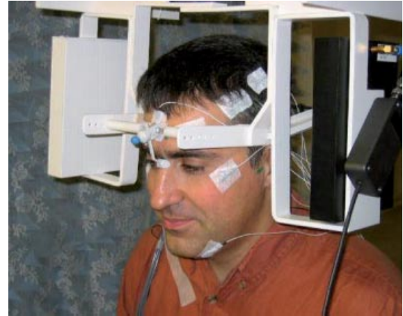
Fig. 1. The exposure situation, a headset with a fixed antenna placed on the left side of the head and a ceramic plate attached to the left ear lobe for heating.
